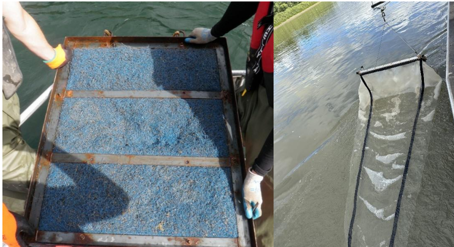
Figure 7.1: Standard egg mat (left) and drift net (right) used to collect embryos and larvae. The tapered plankton net ends with a collection cup device (not shown in the photo) (Photo credits: Egg mat (J. Crossman) and drift net (M. Webb)).
