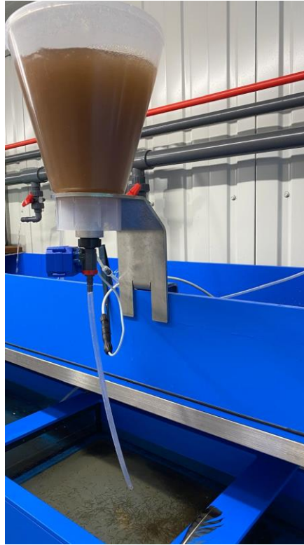
Figure 10.4: Automatic feeders for live feed, e.g. Artemia salina (Photo credit: T. Friedrich)
