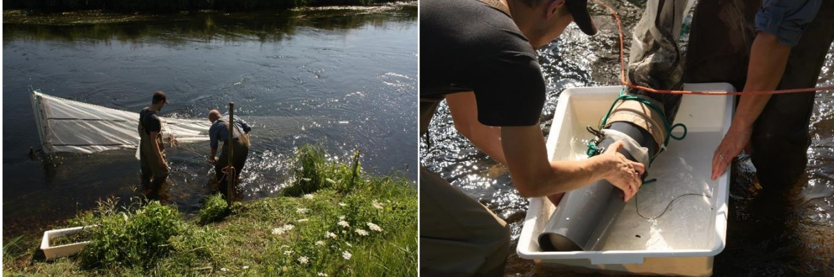
Figure 10: Deployed D-net close to the shore and the opening of the detachable collection bucket into a collection box (© IGB, J. Gessner).
