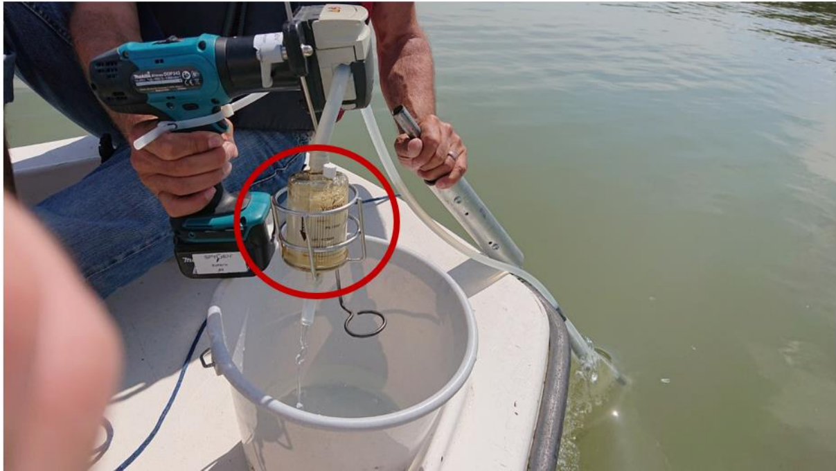
Figure 3: eDNA sample with the sample filter in the red circle. The water flows in the direction of the black arrows (© BOKU, P. Meulenbroek).
