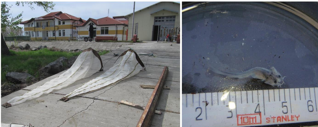
Figure 9: D-nets for larvae and eggs used in the Danube in Romania with an area of 0.44 m 2 , 4 m long and a mesh size of 2 mm (left) and a captured beluga sturgeon larva (right, © DDNI, M. Paraschiv).
