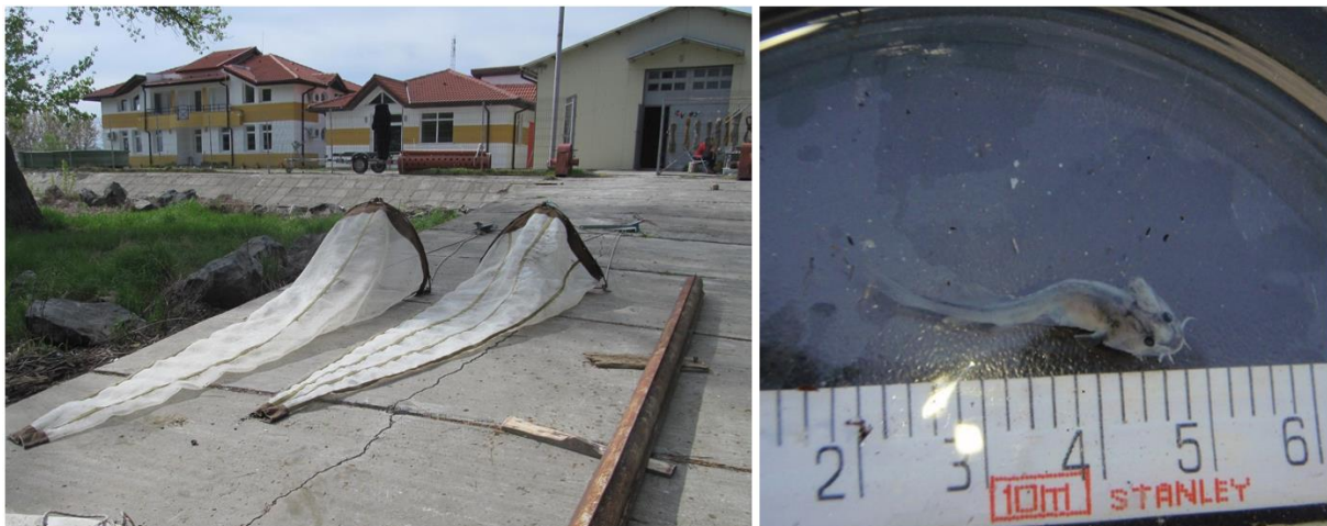
Figure 8: D-nets for larvae and eggs used in the Danube in Romania with an area of 0.44 m 2 , 4 m long and a mesh size of 2 mm (left) and a captured beluga sturgeon larva (right, © DDNI, M. Paraschiv).
