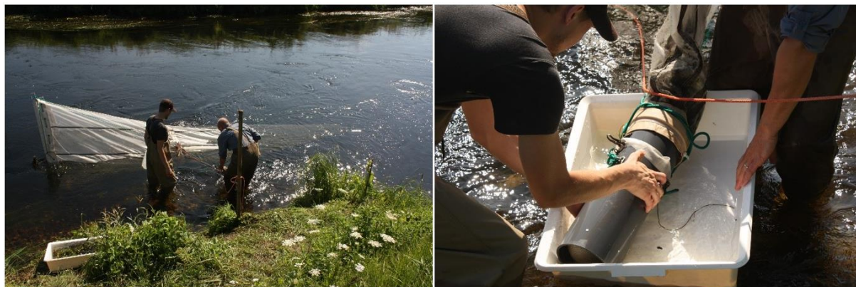
Figure 9: Deployed D-net close to the shore and the opening of the detachable collection bucket into a collection box (© IGB, J. Gessner).
