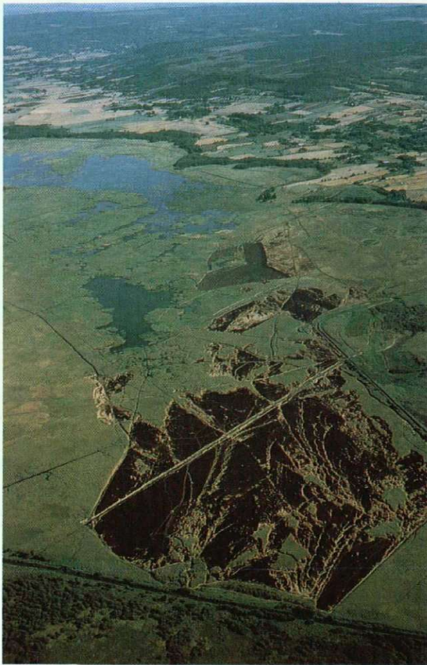
Prior to a rise in the water level, the reed is burned (black areas) and destroyed by means of rotovation (grey areas).
