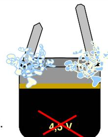
The voltage at the two terminals of the worn-out battery is zero or very low.
