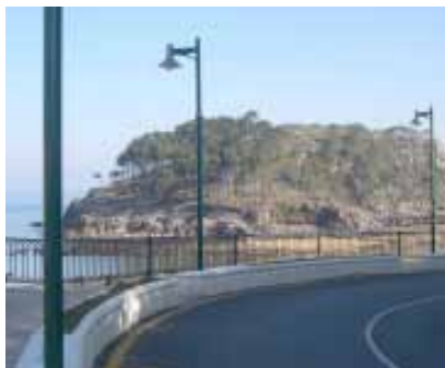
Ills. IV-10 and IV-11: (Left) Footpath separated from traffic lanes by a white parapet, including top landscaping and lights. (Right) The footpath around the road bend includes a scenic viewpoint
