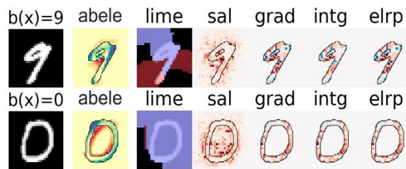
Figure 6. Example of saliency maps returned by different explanation methods. The first column contains the image analysed and the label assigned by the black-box model b of the AI system.
