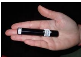
Figure 12: Acoustic tag (© WWF-Bulgaria).
