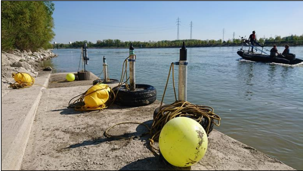
Figure 14: Hydrophones to be deployed as a receiver array ready for setup on the shore below the Freudenau hydropower station (© IHG/BOKU).
