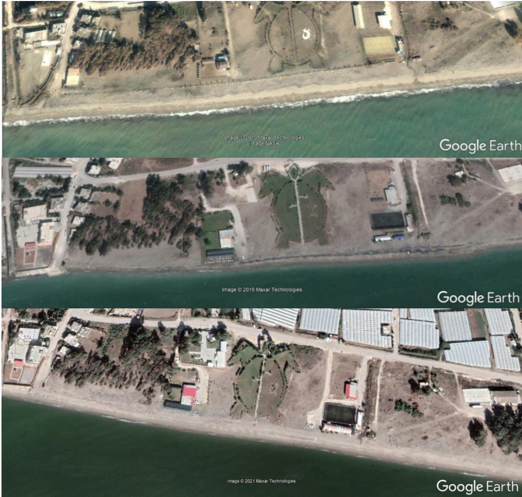
Fig. 37. Kazanlı, Section K2. July 2021. Satellite imagery showing coastal erosion progress. Top: 2007; middle: 2018; bottom: 2020 (Source: Google Earth).
