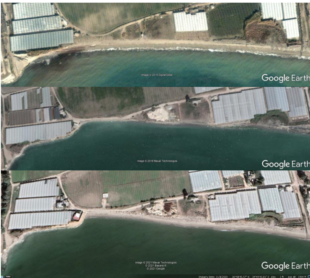
Fig. 36. Kazanlı. Section K3. July 2021. Satellite imagery showing coastal erosion progress. Top: 2007; middle: 2018; bottom: 2020 (Source: Google Earth).
