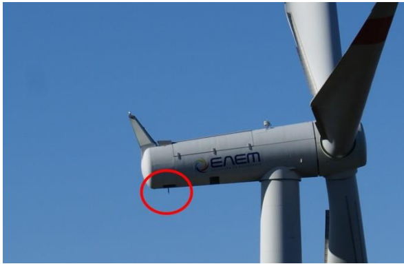
Figure 2 Picture of the microphone at the nacelle at WF Bogdanci, taken from the ground (photo: G. Rnjak)
