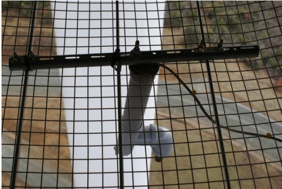
Figure 1 Picture of the microphone at WF Bogdanci taken from inside of the nacelle (photo: G. Rnjak)
