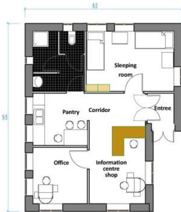
Fig.9.3. Ground floor site offices.
