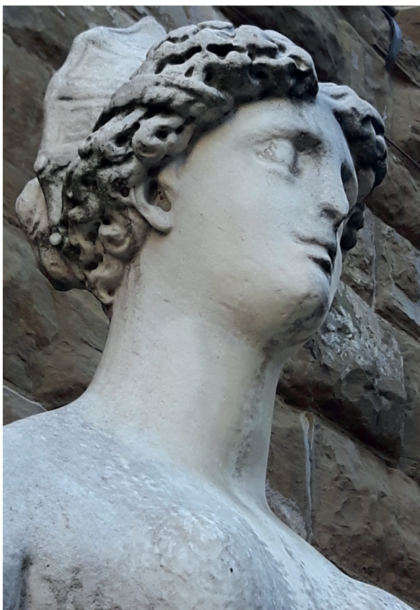
3. - Black, grey and white areas on carbonate stone due to the combined impact of precipitation, gaseous pollutants and carbonaceous particles.
