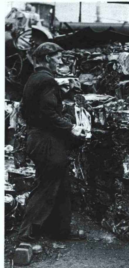
Baled motorcars. Blocks of metal that were once cars being stacked ready for delivery to a steel works for re-use. When a car is retired from use it goes first to a wrecker, who strips it of its valuable parts, and then to a scrap processor who crushes it, bales it, and sells it to a steel mill. The price paid by a wrecker is often less than the cost of transport and for a severely damaged or cannibalized car he may even charge towing costs. Thus the final owner's economic incentive to deliver his car for processing is slight, non-existent or even negative. The rate of abandonment is increasing. In New York City, 2500 cars were towed away as abandoned on the streets in 1960; in 1964 the figure was 25 000; in 1969, more than 50 000.
