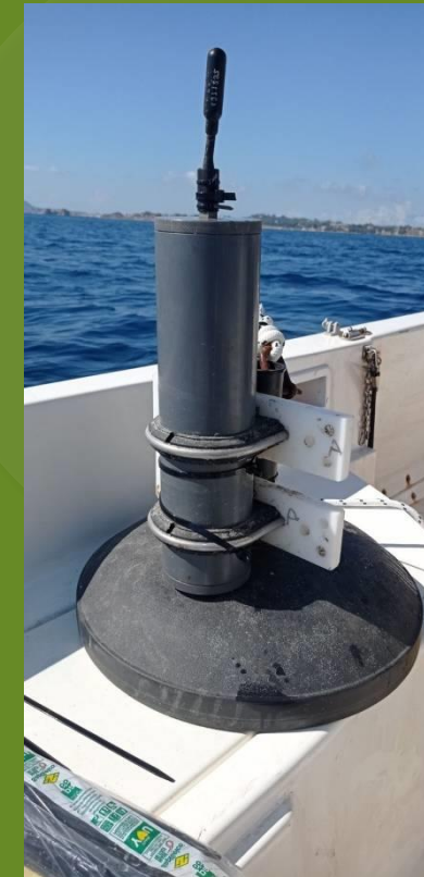
Placement of two underwater hydrophone in Lagana's Gulf for the measurement of noise and its impact on sea turtles
