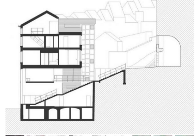
8 - The new access from the gatehouse to the "Minimes" Terraces is a passage under an apartment building, which includes tourist facilities and accommodation.
