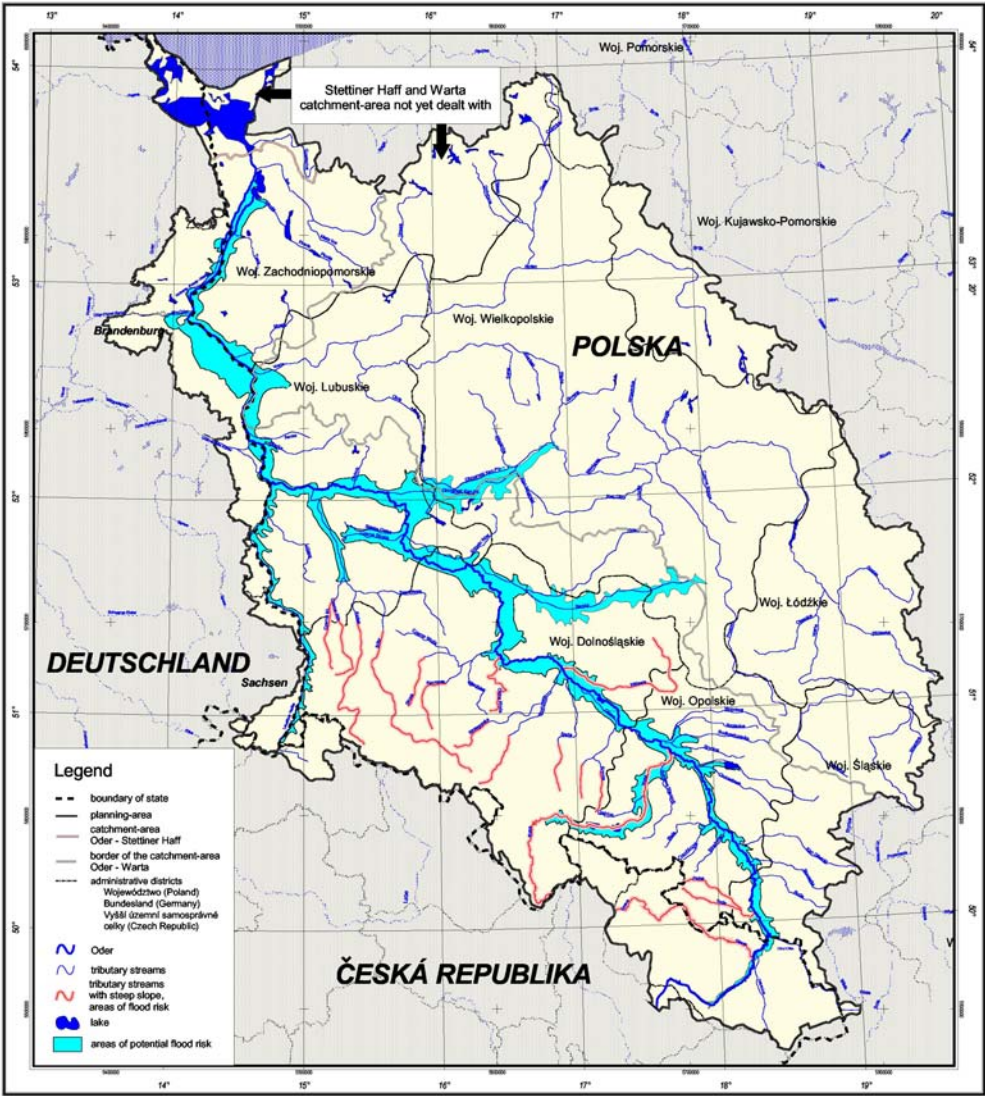
Figure 2 Potential Areas of Flood Risk
