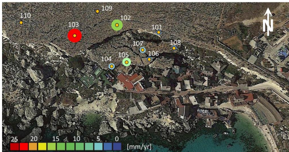
Figure 6: Location of the GPS benchmarks. The size and colour of the circles represent the rate of the vertical deformation. Benchmark 106 has been calculated till the last available measurement of November 2012.
