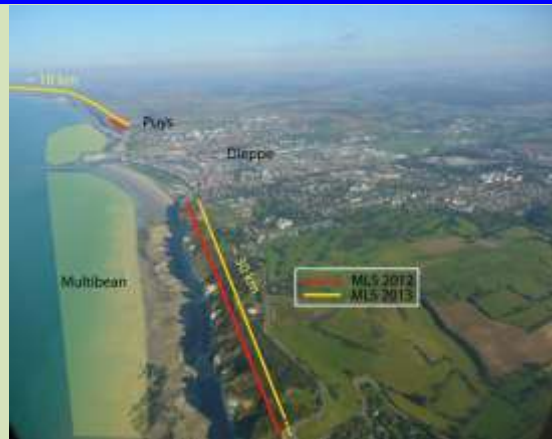
Figure 3.1 Location of the different survey campaigns carried out along the coast in September 2012 and September 2013 from Cap d'Ailly (Pourville) to Puy (Upper Normandy).
