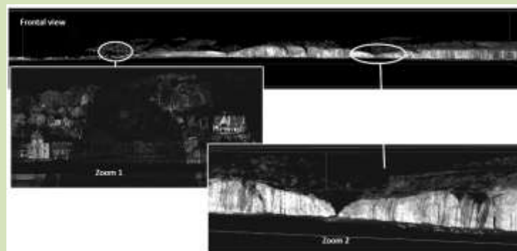
Fig. 19 - Cloud points obtained by MLS (Mobile Laser Scan) from Dieppe to Pourville (Upper Normandy, September 2012) (by C. Michoud, D. Carrea, M.-H. Derron, M. Jaboyedoff, UniL CRET)
