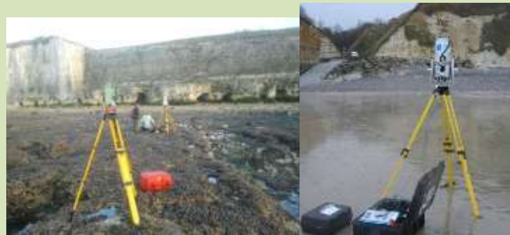
Fig. 22 - TLS (Terrestrial Laser Scan) survey at Puys and Petit Ailly, Upper Normandy
