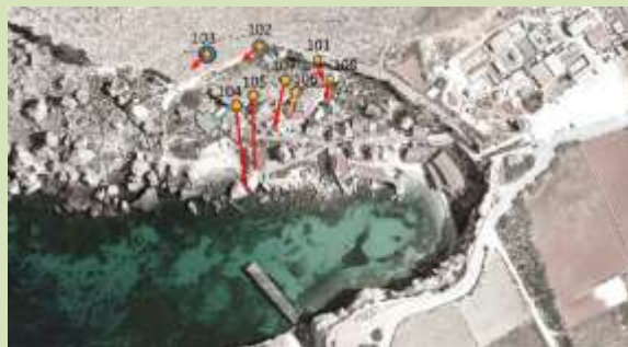
Fig. 9 – Displacements measured at the monitoring site of Anchor Bay, NW coast of Malta. Arrows refer to planar displacements and circles to vertical displacements measured between 2006 and 2013.
