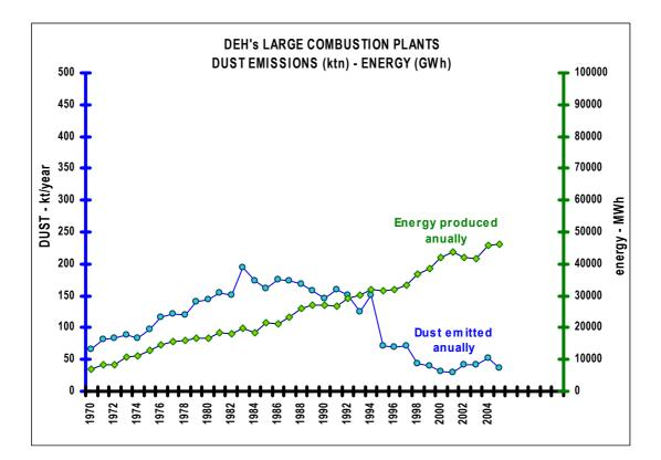
Figure 1: Dust emissions reductions versus increase in energy production from DEH's LCPs, due to pollution control measures imposed on them.
