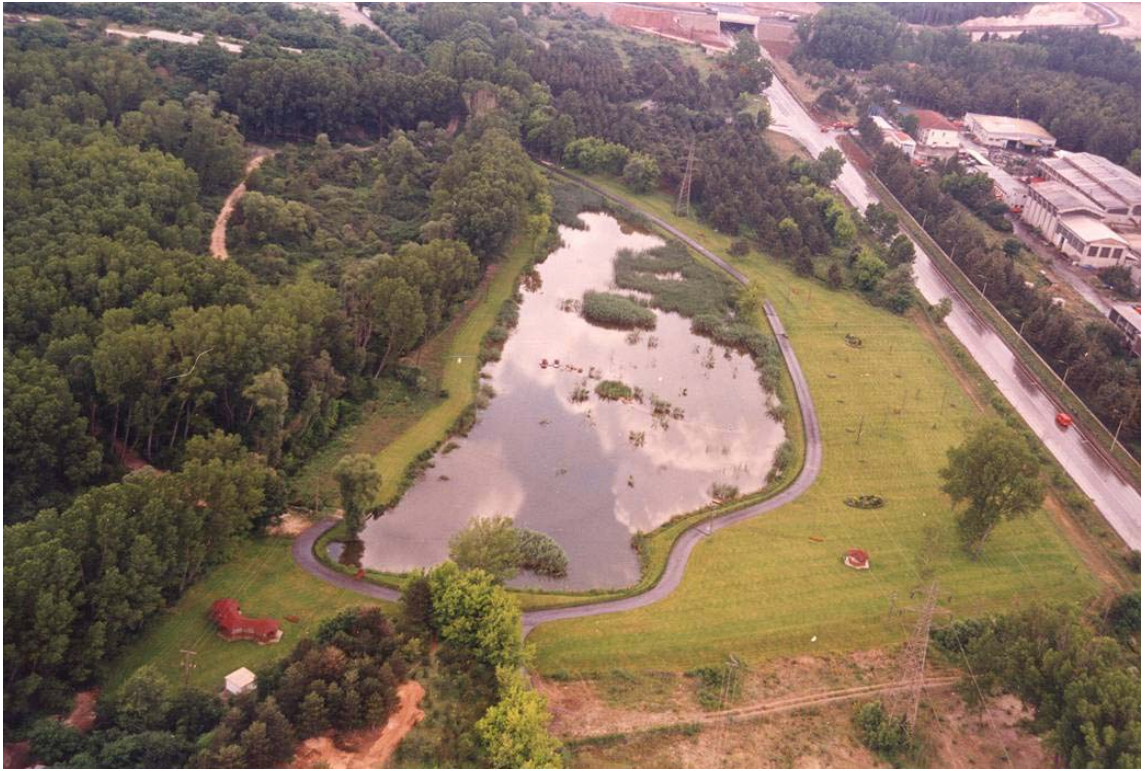
Figure 1: Artificial wet-land in West Macedonia Lignite Centre created in exhausted mines
