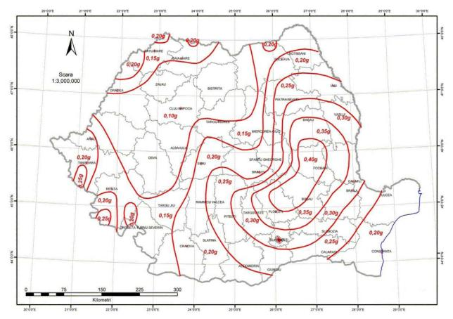
Seismic Zoning Map Code P100-1/2013 for Seismic Design. Return period 225 years. Bucharest – design acceleration 0.3 g
