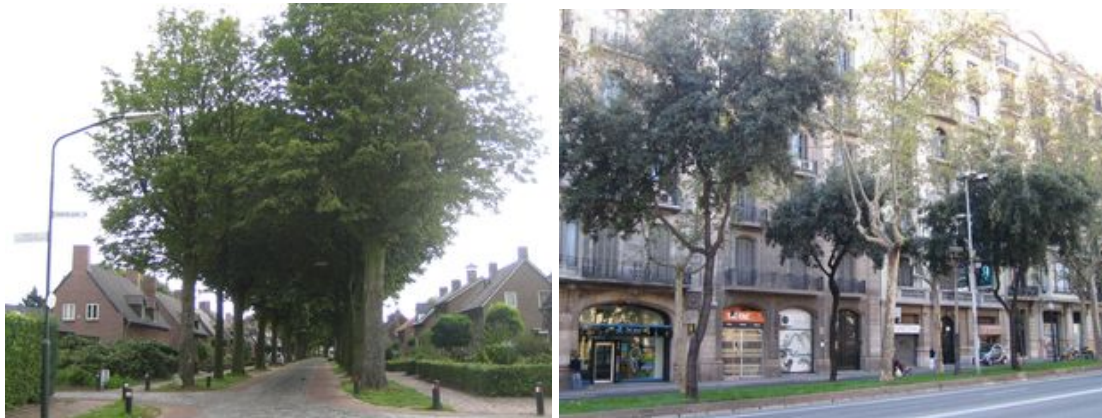
Figure 48: An arrangement in the spirit of the Dutch “Sustainable Safety” programme: trees are used to keep pedestrian walkways separate from cars. Figure 49: A double row on a central reservation in Barcelona.
