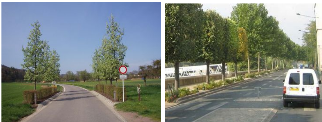
Figure 62: A double row of trees set in a low clipped hedge signals the approach to a built-up area in Luxembourg. Figure 63: Alongside the Seine, near Paris, a sequence of clipped lime trees takes the place of free-growing plane trees. The change visually signals an intersection, is aesthetic, and also acts as a safety barrier to stop disease spreading in the event of an outbreak of canker stain.
