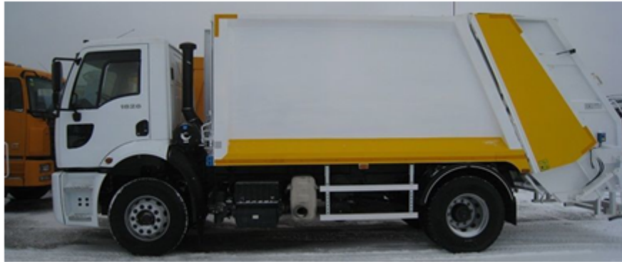
Figure 9 Example for a compaction truck with 10 Mg capacity
