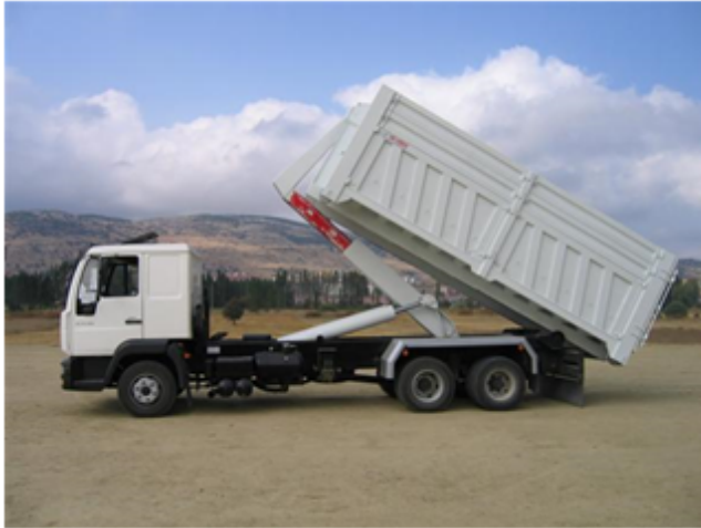
Figure 8 Example for hook lift truck for long distance transportation
