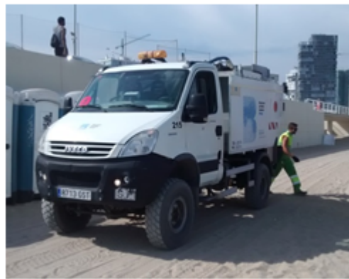
Figure 6 Example for 1.1 m 3 steel container (left) and small 4x4 compaction truck (3 Mg capacity) (right) for waste collection
