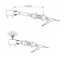
In instance where the conductors Suggested practices: run above or too close to the crossarm, (c) tubing should be used. Junction power poles should be treated in the same way (insulation of conductors which come too near to a perching site closer than 60 cm).
