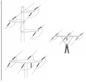
Strain poles with one conductor above the crossarm. Risk high (see also Fig. 3):
