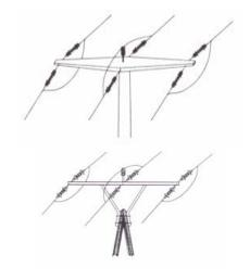
Bird-safe strain poles require insulating chains at least 60 cm in length. Hazardous constructions can be mitigated by (a) lengthening the chains or (b) installing perch rejectors (upright "whisk brooms") on the crossarms.
